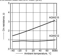
2.-(2) On resistance vs. ambient temperature characteristics
